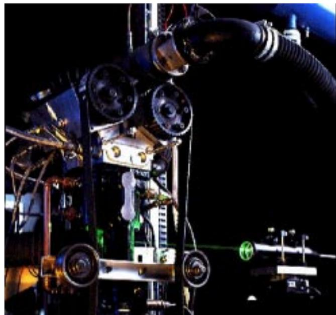
Figure 4: Typical single cylinder Ricardo "Hydra" optical research engine
