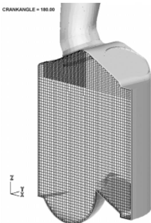
Figure 1: CFD Surface geometry and computational mesh
