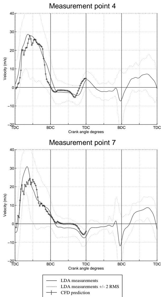
Figure 8: Comparison of CFD air simulation and LDA results
