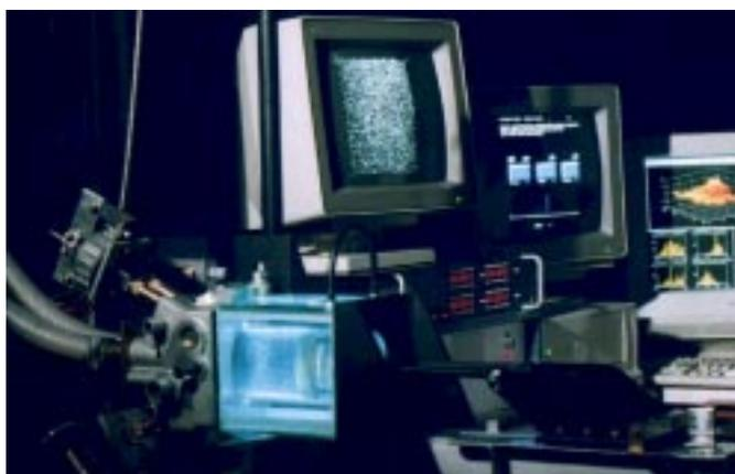
Figure 3: The dynamic flow visualisation rig
