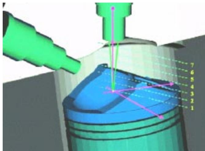
Figure 5: Measurement locations reached via the spark plug probe
