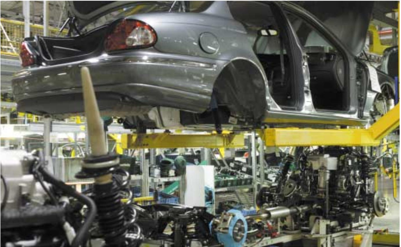
**A powertrain is installed into a 2.0D X-TYPE at Jaguar's Halewood plant**
