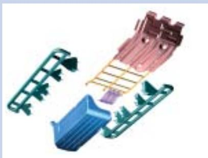
**Structural analysis was used to design rocker tubes strong enough to support the whole vehicle weight without damage**
