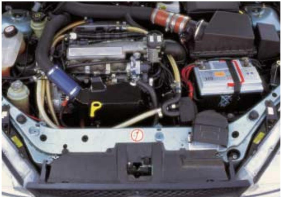
**Downsized 1.1 litre, three-cylinder LBDI® engine in Focus demonstrator matches drive characteristics of standard 1.6 – but with a 20 per cent fuel saving**
