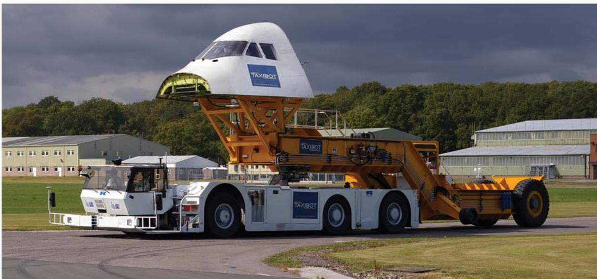
***The IAI TaxiBot demonstrator vehicle designed and built by Ricardo, shown coupled to its Ricardo designed hydrostatic dynamometer equipped test trailer capable of simulating the taxiing performance of a large passenger aircraft***
