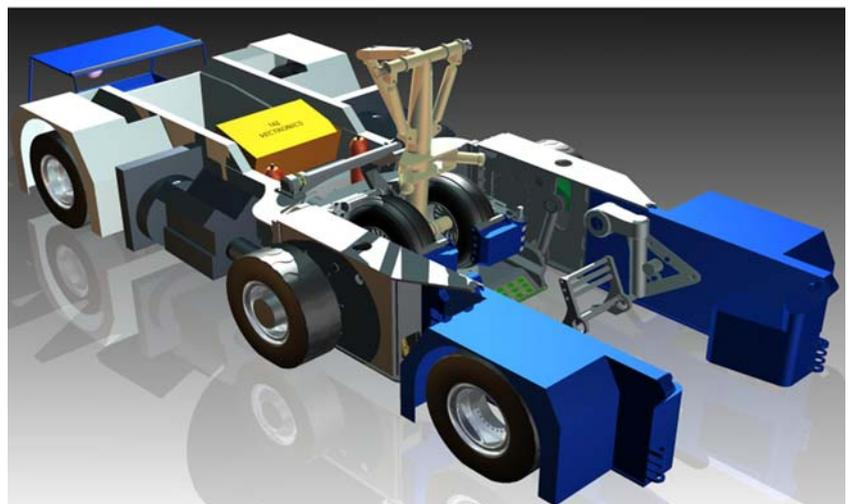
*CAD model of the TaxiBot showing aircraft nose wheel and landing gear fully engaged*
