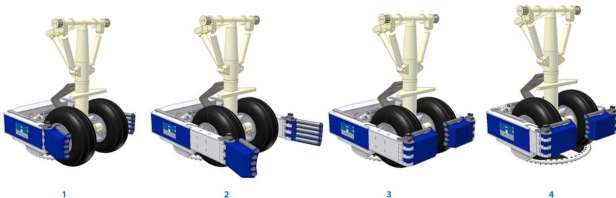
***On engaging with the TaxiBot, the nose wheel of the aircraft enters the vehicle turret and is quickly clamped securely into position. The turret is able to rotate freely and can hence take steering and braking requests directly from the nose wheel - the flight crew can thus manoeuvre the aircraft around the taxi-ways of the airport without using the plane's main engines***
