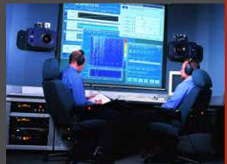
target sounds. WAVE is also used to develop the muffler system and to modify the sound to match the targets. This modelling phase can involve hundreds of iterations, of which perhaps two or three will be built and fitted to production motorcycles.
